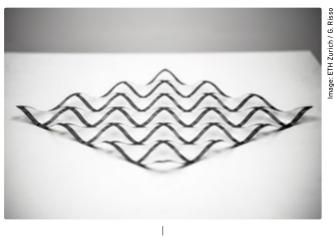
Lightweight and easy to produce, the multistable structure can be flexibly expanded and reshaped as required.
