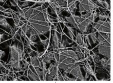
Electron microscope images show significant colonisation and degradation of the polymers by fungi and bacteria after just six weeks.
